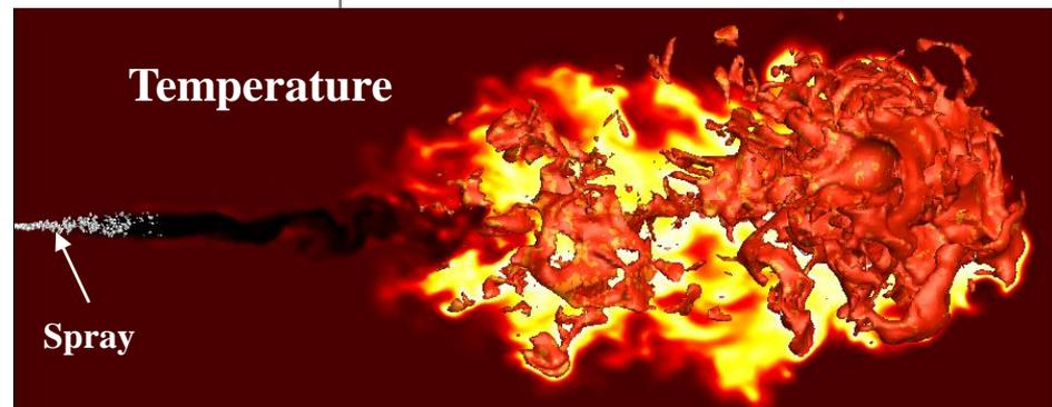
Flame Starts in Spray Generated Turbulent Zones at Tip of Fuel Vapor Jet
