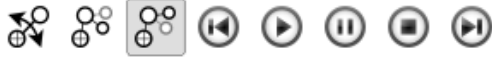
FIGURE 6. Post synthesis options; from left to right: switch actuated dyad, crossed configuration, open configuration, step backward, play, pause, stop, step forward
